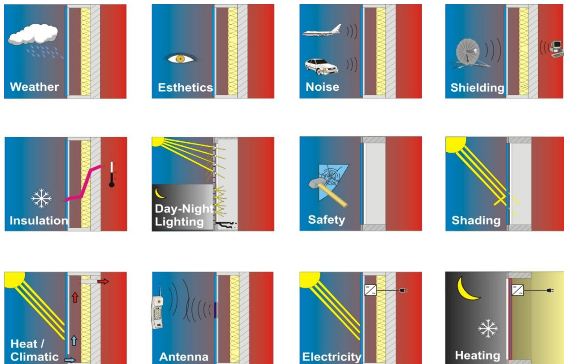
Figure 1. Multiple functions of PV modules. Source: Multielement project
